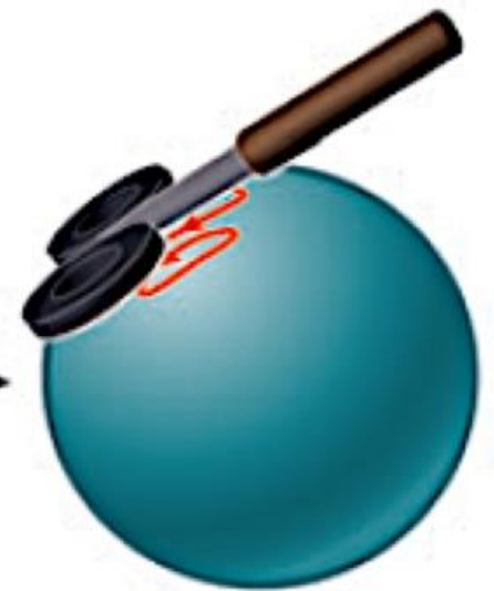
Induced current in conductor
